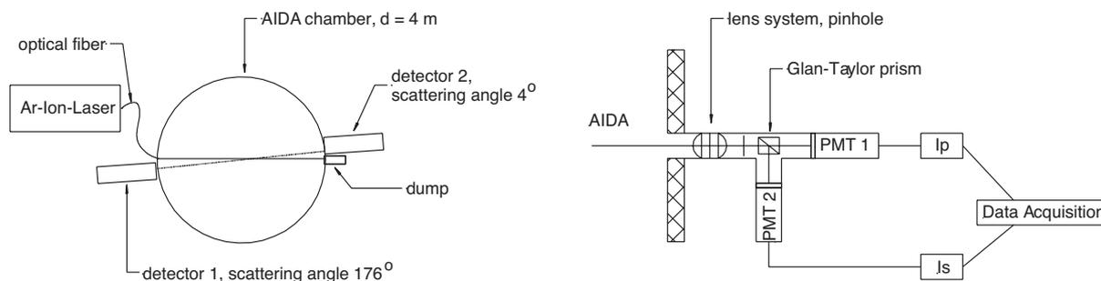
Fig. 3 Overall cross section of the laser scattering device (left) and detail of the detector for measuring backscattered light intensity and depolarisation.
