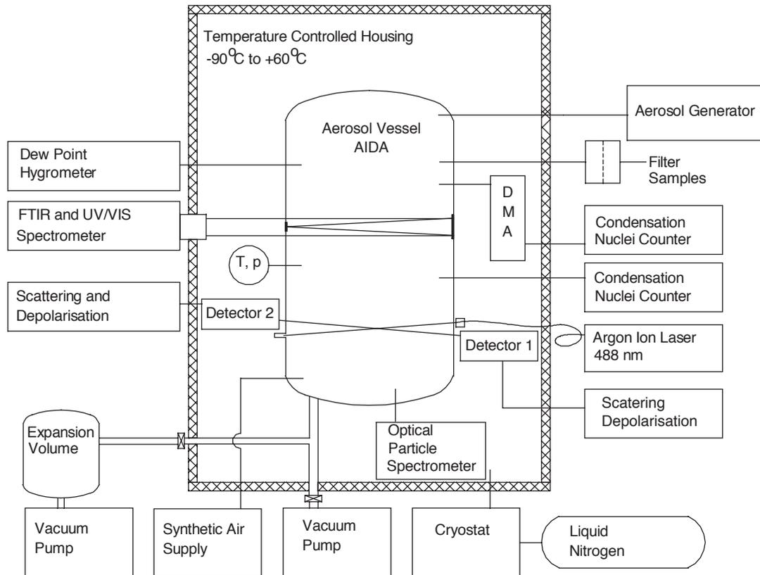
Fig. 1 AIDA main components and instrumentation available for ice activation experiments.
