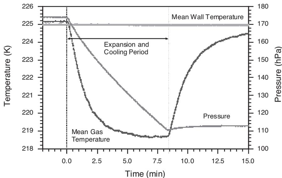
Fig. 2 Time profiles of pressure, mean wall temperature, and mean gas temperature during a typical ice activation experiment.
